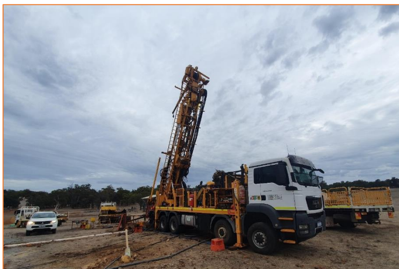
Figure 4. Chalice Gold Mines' diamond drilling activity in progress at the Julimar Project
